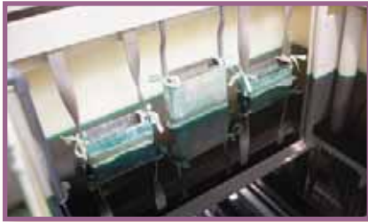
Figure 3. A typical Watts nickel bath setup.
