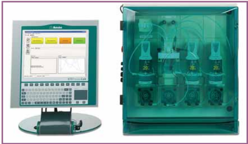
Figures 5 & 5a. Rendering of an analyzer that is closely integrated with the plating process
